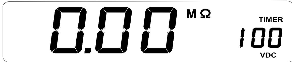
Press SELECT to check the preset time. The LCD screen display TIMER, PRES is shown on primary display, the secondary display shows the preset time. Press ENTER, the meter display Set. The time can be adjusted by  $\Delta/\nabla$  button.
