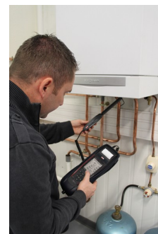
Ambient CO checking
